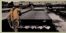
Hollow-core, pre-stressed concrete panels
